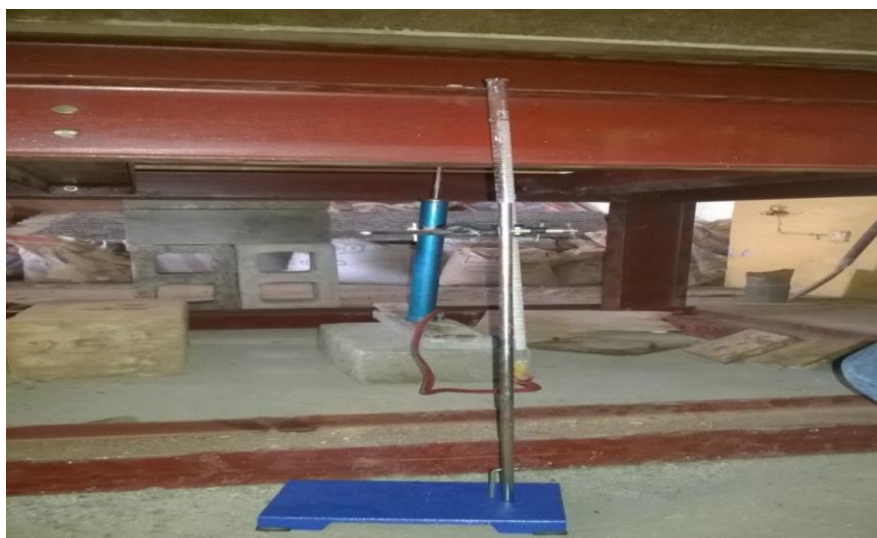
Plate 4.2: Deflection measurement using principle of incompressibility of water
